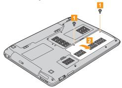
**6** Remove the frame fixing screw.
